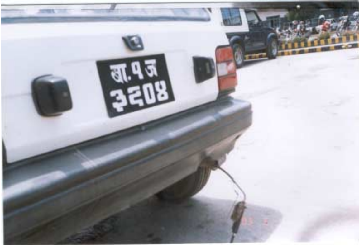
Figure 3.5 Incorrectly inserted probe into the tailpipe
