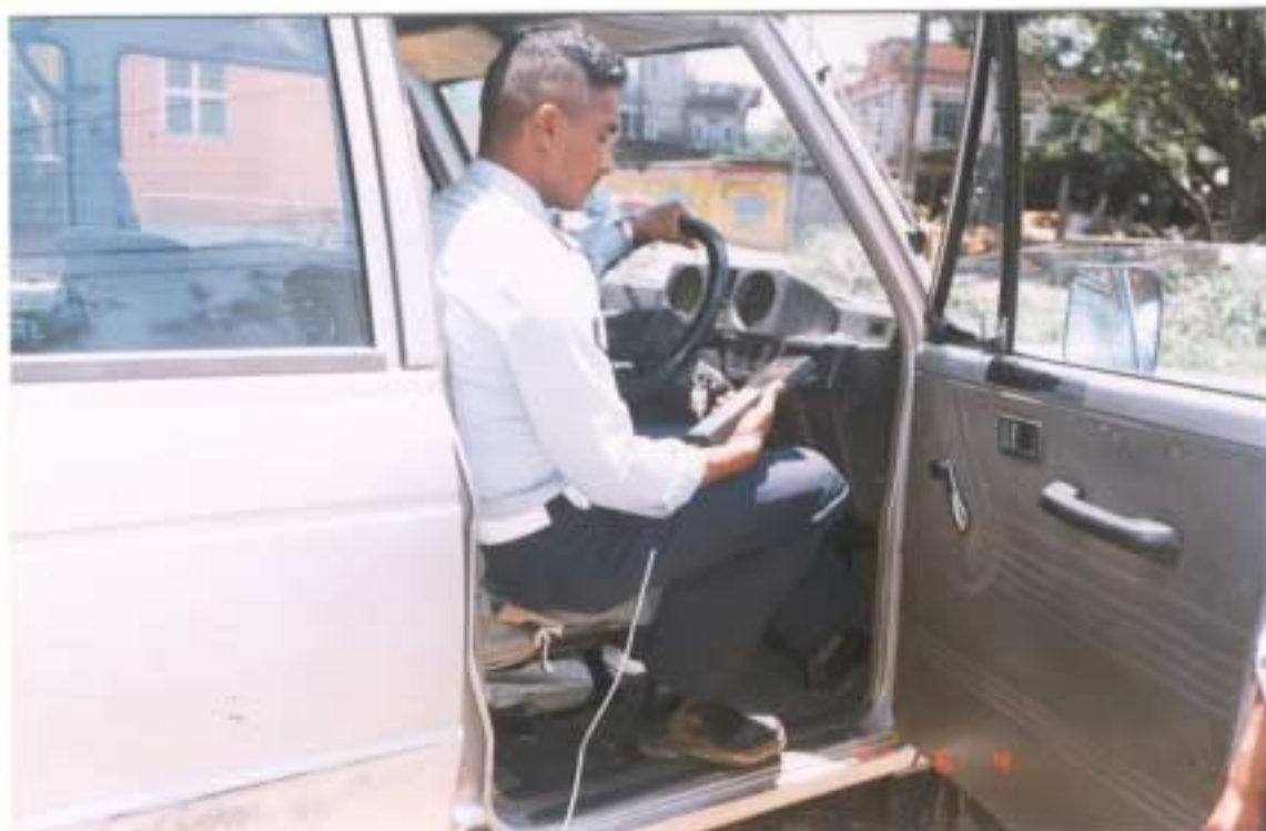
Figure 3.2 Measuring smoke opacity from diesel vehicle at Satdobato, Lalitpur
