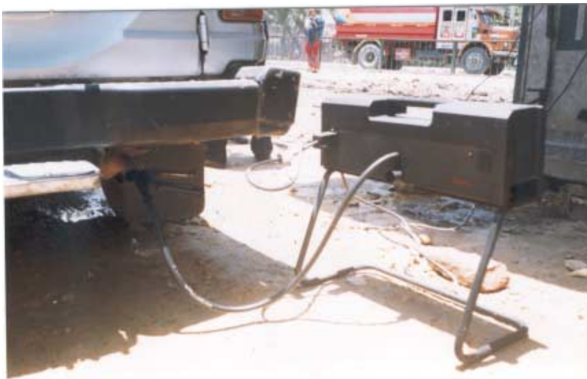
Figure 3.1 Insertion of probe into tailpipe of diesel vehicle
