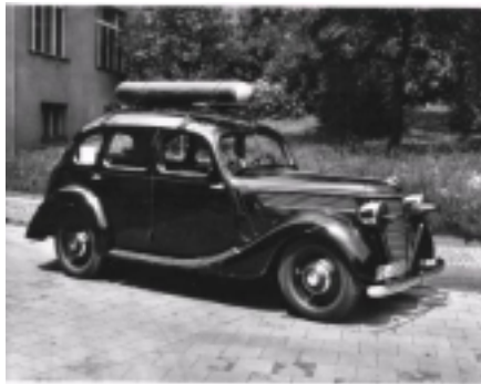
Czech passenger car Wikov running on compressed town gas – around 1936
