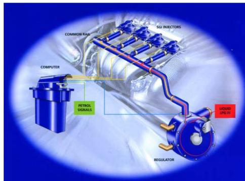
Moving from the 1980's vintage carburettor fuel mixer, to the latest computer-controlled, sequential multi-point injection systems (see illustration above), the new generation of LPG cars embody a degree of sophistication that is the equal of any comparable petrol vehicle. Precise control over the timing and amount of fuel injected provides a quantum improvement in emissions and a significant fuel consumption benefit. Many of the new LPG fuel systems are already certified to Euro 4.
