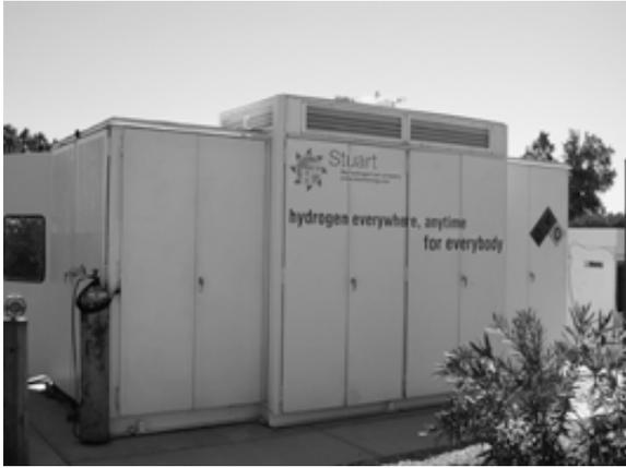
**Figure 4. Stuart Energy's modular compressed hydrogen station**
